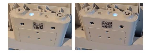
The unit will then beep 5 times followed by a further sequence of flashing lights. Then after approximately 30 seconds the unit will beep a further 5 times and both lights will be steady. The unit will then beep a further 5 times and a green light will display to indicate the reset is complete (see below).
