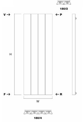
Wall to front face = 110mm Wall to pipe centre = 25mm
