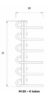
**TECHNICAL INFORMATION** STANDARD CONNECTIONS 1/2"  $\mathbf{F} = \text{Flow } \mathbf{R} = \text{Return } \mathbf{P} = \text{Plug } \mathbf{V} = \text{Vent}$
