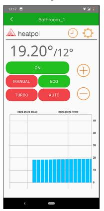
The first temperature (  $19.20^{\circ}$ ) - is measured with the remote / temp. sensor (H+R). This is the actual room temperature. The second (  $12^{\circ}$ ) is the temperature set for the room.
