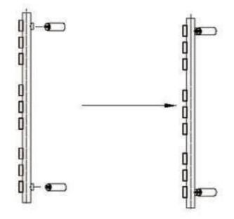
Step 4: Fix the brackets to the wall with screws.
