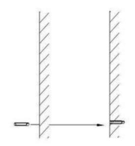
Step 2: Pinpoint the positions on the wall then drill four accordingly, and fix the wall plugs into the wall.
