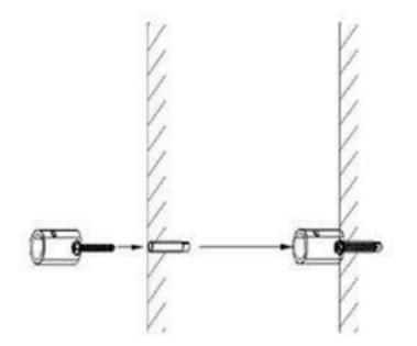
Step 3: Connect the bracket socket to the wall with screws.
