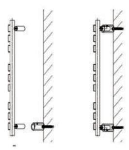
Step 5: Mount the towel rail to the wall and tighten the screws in the brackets.
