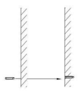
Step 2: Pinpoint the positions on the wall then drill four accordingly, and fix the wall plugs into the wall.
