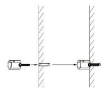
Step 3: Connect the bracket socket to the wall with screws.
